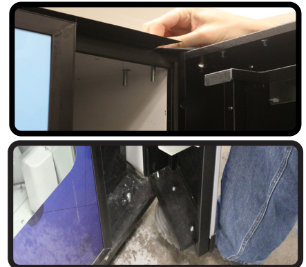
4.C) Lift the OEM door off the cabinet bottom hinge and set aside.
