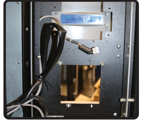
1.B) Disconnect and remove any payment systems currently in the door, set aside for future use.
