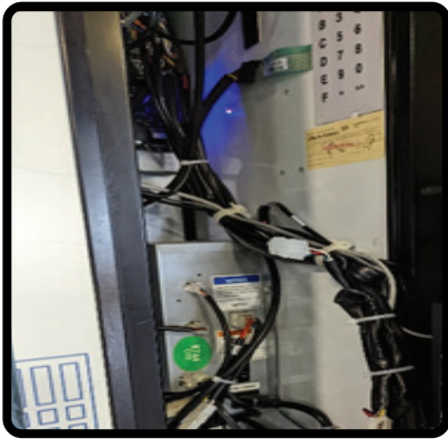
3.A) Disconnect all Harnesses and the Ground Wire connecting the OEM door to the cabinet.
