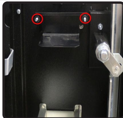
2.A) Remove plastic OEM board cover, exposing the board underneath. Remove the two nuts securing the electronic housing bracket, then remove the bracket so that it can be installed later onto the new door.
