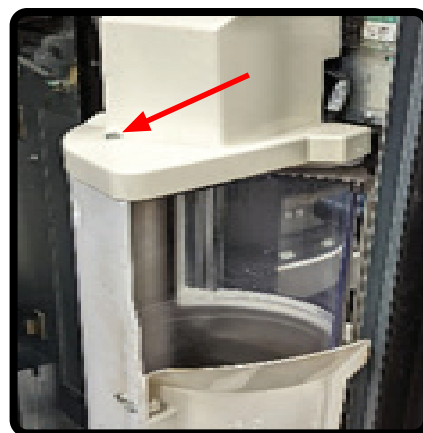
2.B) Remove screw on top of the OEM delivery port marked in the picture above. Remove the upper housing to reveal the screws that are used to secure the OEM delivery port to the door.
