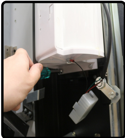
3.D) Secure the bottom of the OEM delivery port and turret electronic housing bracket to the bottom delivery port mount with (2) nuts.
