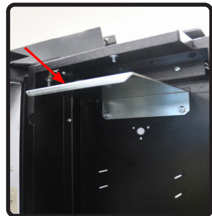
3.H) If the door switch doesn't match the one in step 3.F, install switch contact bracket (VE1019552) instead.
