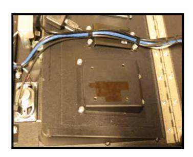
**3.**) Unplug the USB (**VE1015711**) cord from the Ingenico reader. Next remove the 4 screws indicated in the picture. Ensure you leave one hand holding the Ingenico reader as it will fall out once released.
