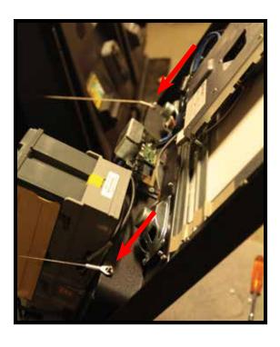
1.) Unlock kiosk and lower front door. Remove the Nuts holding the door up as shown in the image above.
