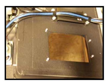
4.) Remove the 4 nuts as shown in the picture above. This will allow you to remove the Ingenico bracket.
