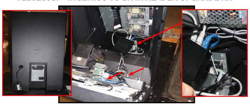
**9.)** Remove the grommet from the back of the kiosk and insert the Switch Power supply into the kiosk cabinet, then connect to the Switch. Connect the preexisting Ethernet cable from the screen into the Switch.
