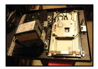
**2.**) Once the door is detached, Lay it flat on some sort of cushioning. This will allow the door to lay flat without damaging the screens.
