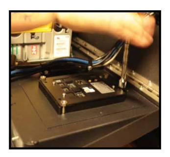
7.) Using the Hex mounting adapters (MEI250031081P) secure the castle reader to the kiosk using the 11/32 Nut Driver. Secure each mounting hex before tightening all the way. This will ensure it is secured properly.
