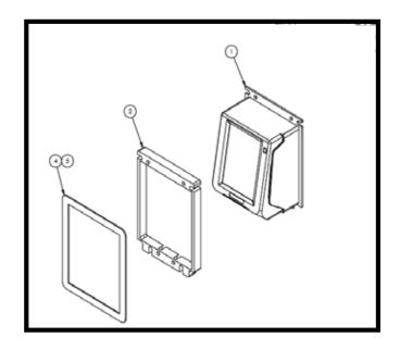
**6.)** Secure the New castle Spacer over top of the Castle reader. Insert into the Kiosk so that it can be secured in the next step.
