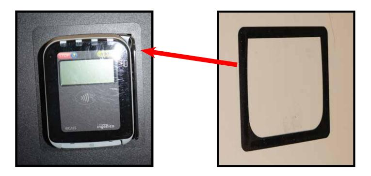
**5.**) In order to secure the new castle Lynk reader you will need to remove the old bezel. This is being held on with double sided tape, if necessary use a tool for removal.
