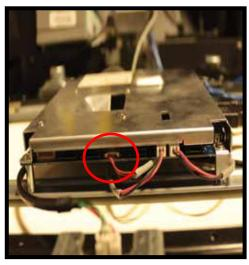
**8.**) First plug in the USB ( **VE1015711**) that was with the original parts. Then Plug in the castle Harness into the back of the castle reader into the designated port. Once connected insert the loose end of the harness under the screen as shown in the picture above. Lastly secure the Harness into the third port on the screen, as circled above. Use a tool if necessary.
