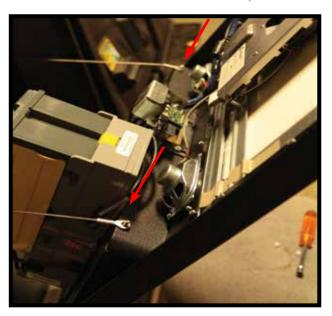
11.) Lastly raise the Kiosk door and secure the arms onto the studs indicated in the Picture. Secure the nuts that you removed earlier. Door is now ready to be closed and Locked.
