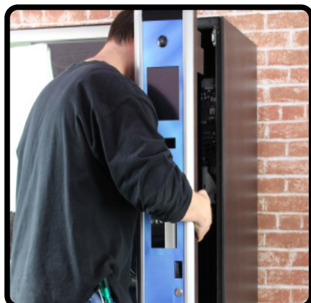
2.D) Hold door in vertical position and stand up to hold the door near the top.
