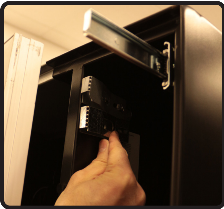
2.A) Check the LOCK BRACKET (VE1017104) already secured to the cabinet against the one included in the kit. If the width on the new one is equal to or smaller than the old one, no need to replace. If not the case, replace with the included wider LOCK BRACKET (VE1017104).
