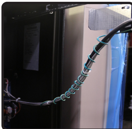
2.B) Wrap the loose end of the ground wire around the preexisting bundle. Feel free to use cable ties if Preferred.
