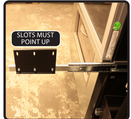
2.C) Install MOUNTING PLATE (VE1019478) to lower left rail using three (VE7207K) nuts. Ensure slots face up.
