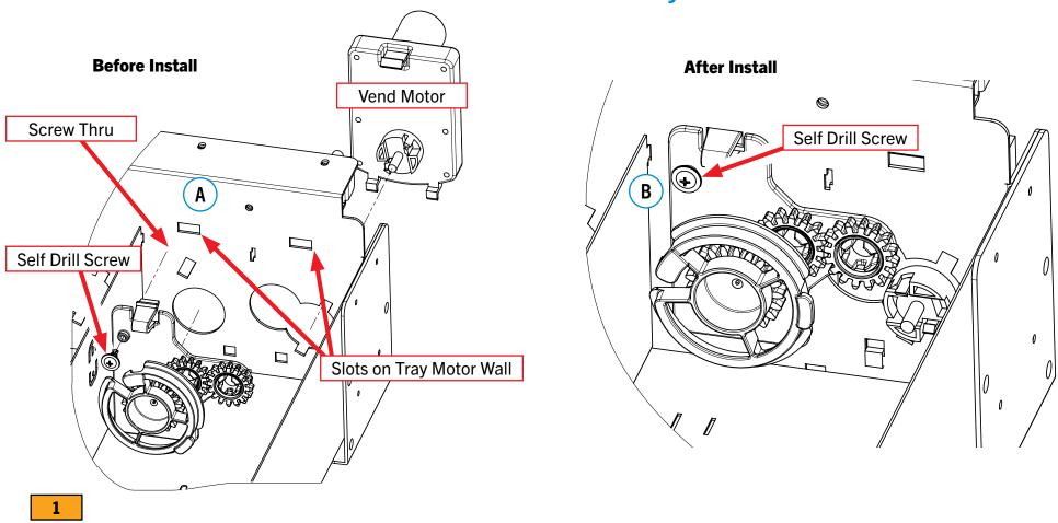
First, insert **Backing Plate with Gears (VE106272)** into the slots in the tray motor slot as shown **(A)**. Using the **Self-Drilling Screw (VE9323B)**, hold the backing plate in position while installing the screw as shown **(B)**.
