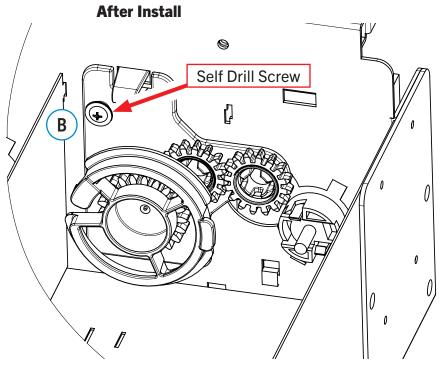
First, insert Backing Plate with Gears (VE106272) into the slots in the tray motor slot as shown (A). Using the Self-Drilling Screw (VE9323B), hold the backing plate in position while installing the screw as shown (B).
