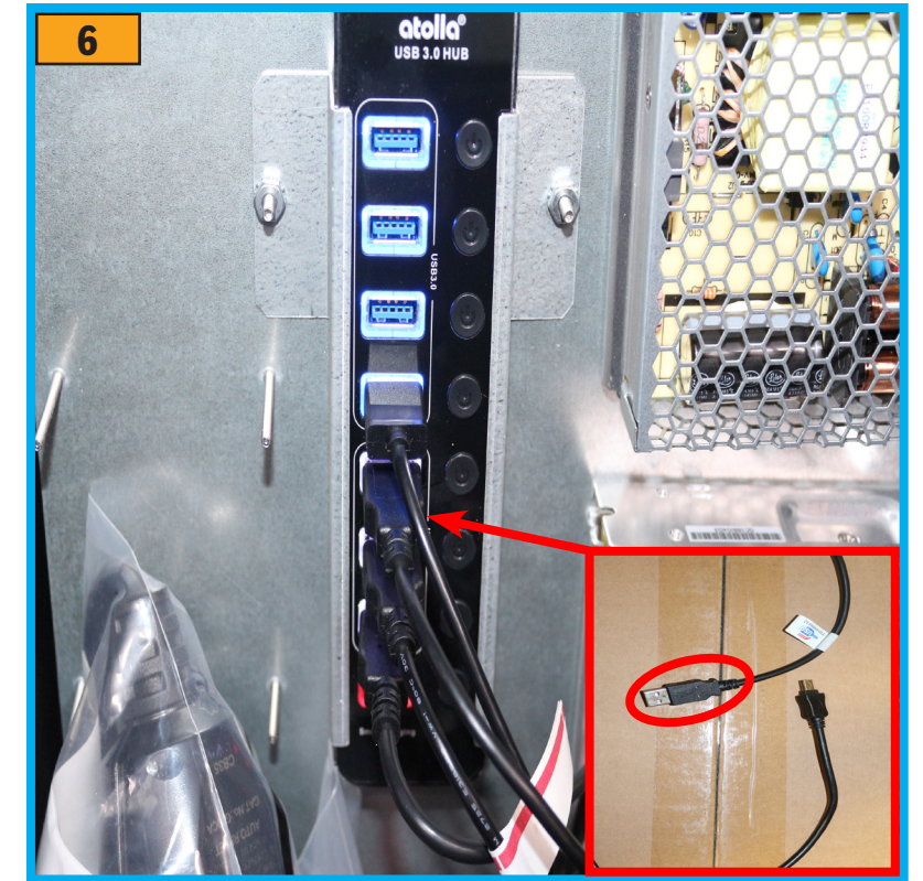
6.) Plug the USB side of the USB 3.0 cable and plug it into the USB port on the USB hub.
