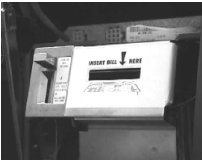
Figure 5 View of Slider Bracket in place with label.
