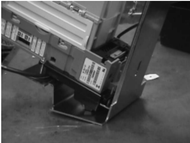
Figure 4 Mounting validator to slider bracket
