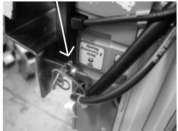
Figure 6 Attach the green/yellow grounding wire to the stud of the slider bracket
